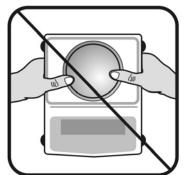
When moving the scale do not press or apply force onto the scales pan!
