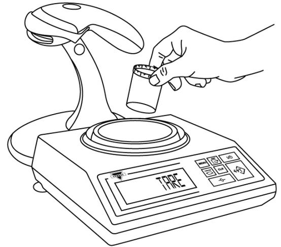
2. Place an empty vial or counting container on the pan. The container's weight will be displayed. Wait for the weight to stabilize and press the T key to tare.
