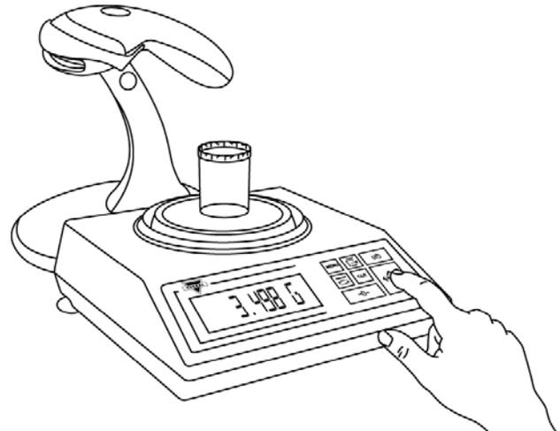
3. Once the scale has finished taring "S-c-A-n b-o-t-t-l-E" will appear on the display indicating you should scan the NDC code associated with the drug.
