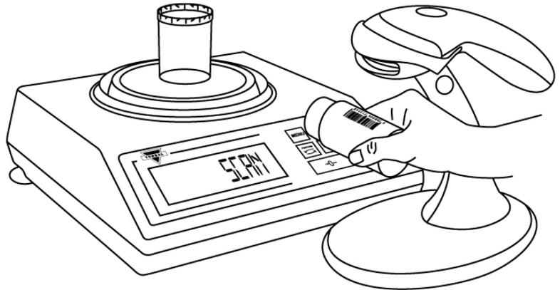
**Note: If Rx Verification has been enabled, the bottle NDC and Rx NDC label must be scanned to allow the scale to check whether there is a match between the two codes.**
