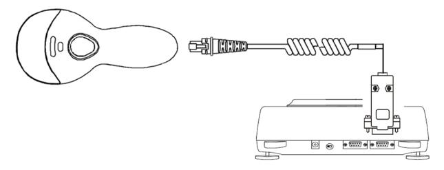
Note: Do not plug in a power adapter to the scanner. The scanner is powered by the scale. Plugging an external adaptor will damage the scanner.
