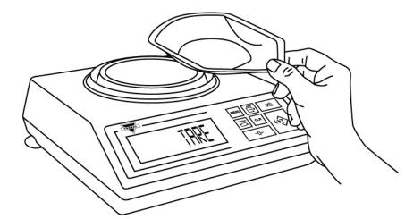
3. Place an empty container on the pan. The container's weight will be displayed.
