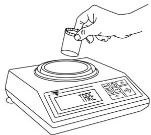
3. Place an empty vial or counting container on the pan. The container's weight will be displayed. Wait for the weight to stabilize and press the T key to tare.
