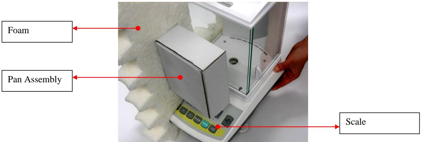
**- Never Ship or Transport the Scale with Pan Components Inside of the Weighing Chamber! -**
