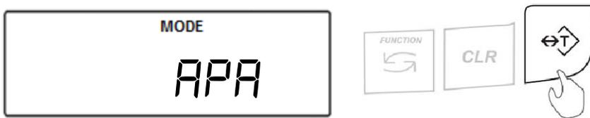
3. Enable APA by choosing either the “2 STOP” approach or the “3 STOP” approach. Confirm the selection by pressing the T key.
