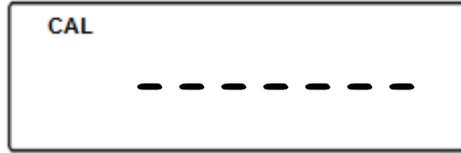
8. When prompted, load a calibration weight equal to the weight displayed on the screen. (Calibration weight varies by model).
