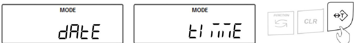
4. Choose “On” to include the field or “OFF” to exclude the field. To confirm the selection press the T key.
