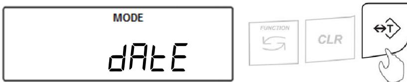
3. Press the T key to scroll between the month and then the day. Press the Function key to increment a digit.
