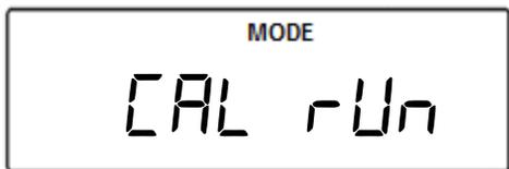
4. During calibration the scale will display “CAL t”. When calibration is finished the scale will return to weighing mode.
