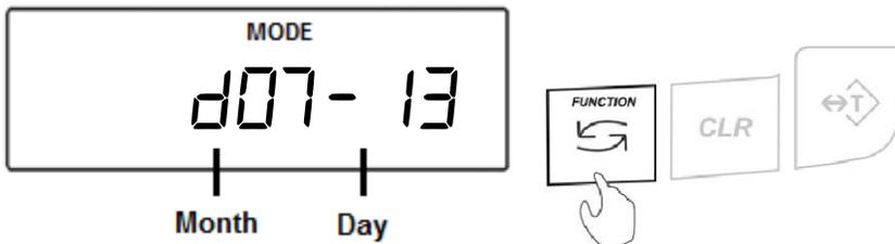
4. Once the day and month are confirmed the screen will switch to the year. Press the T key to scroll between the digits and press the Function key to increment a digit.
