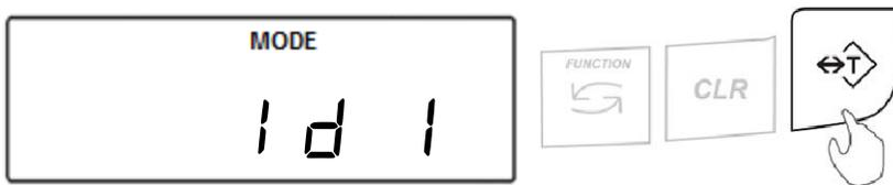
2. Press the T key to add a digit. Press the Function key to increment a digit.
