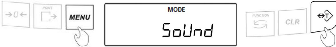
2. Select “On” to enable the sound or “OFF” to disable the sound. To confirm the selection press the T key.
