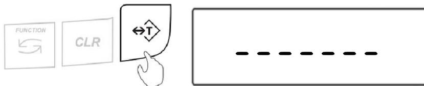
3. When finished clearing the tare, the scale will return to Weighing Mode.
