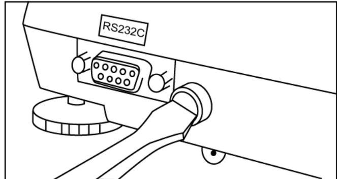
**Warning: Do not attempt to screw the flush sealing screw all the way in. Stop when the screw is flush with the casing of the scale.**
