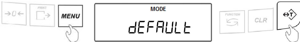
2. Select “YES” to restore the default settings or “nO” to continue with the current configuration. Confirm the selection by pressing the T key.
