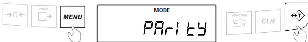
8. Choose the parity type to be used (“nonE”, “odd”, and “EuEn”). To confirm the selection, press the T key.
