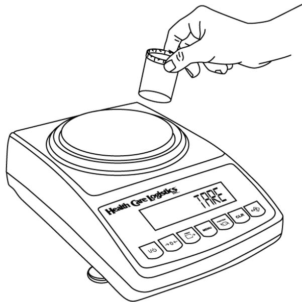
3. Place an empty vial or counting container on the pan. The container’s weight will be displayed. Wait for the weight to stabilize and press the T key to tare.
