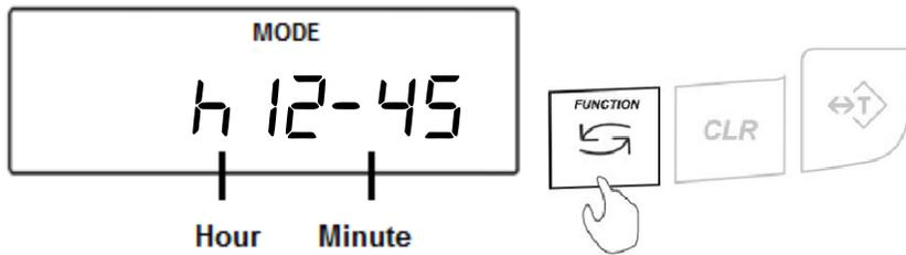
4. Once the minutes and hours are confirmed the screen will switch automatically to the time of day selection. Select “A M” or “P M” by pressing the T key.
