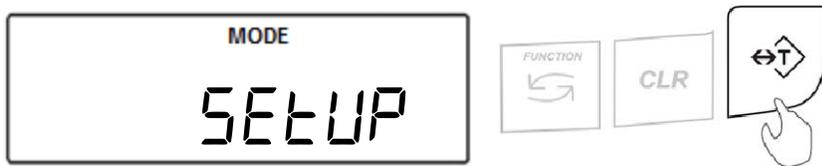
3. Select a field to configure. Confirm the selection by pressing the T key.
