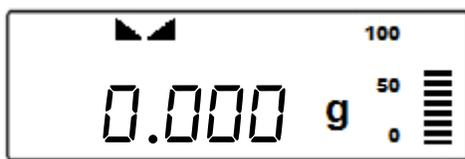
3. When weighing, always place the mass in the middle of the pan. The weighed result may be taken when the stabilization indicator reappears on the display.
