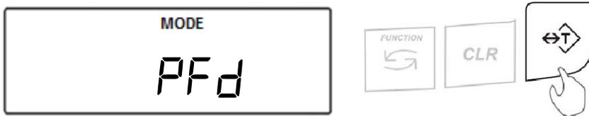
3. Enable PFD by selecting “On” or disable it by selecting “OFF”. Confirm the selection by pressing the T key.
