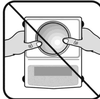
When moving the scale do not press or apply force onto the scales pan!
