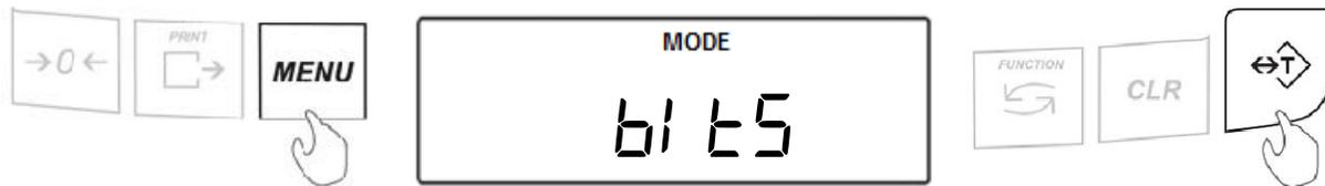
6. Choose “7 bit5” or “8 bit5”. To confirm the selection, press the T key.
