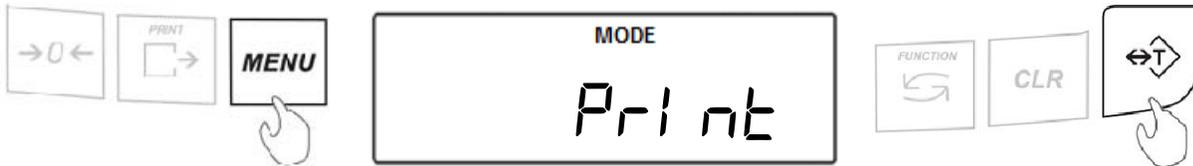
2. Choose the method of printing by selecting either "Auto" or "button" by pressing the T key.
