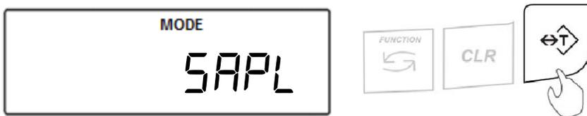
3. Choose the sample size that will be used to establish an average piece weight (**Options are 10, 30, 60, 90, and 100**). To confirm the sample size press the T key.
