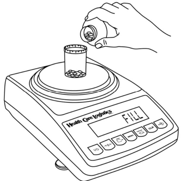
Note: If more pieces have been placed into the container than actually desired, you may use tweezers, a pharmacy spoon, or a similar instrument to remove the container from the pan, dispense out the excess pieces, and place it back on the pan to recheck the count
