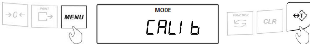
3. Select “CAL rUn” with the T key. The scale will then begin to perform calibration.
