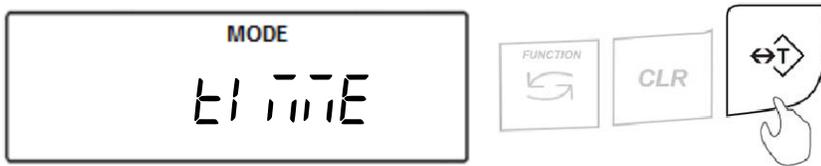
3. Press the T key to scroll between the minutes and then the hours. Press the Function key to increment a digit.
