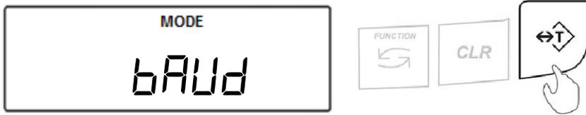
4. Choose the baud rate to be used (“1200”, “2400”, “4800”, “9600”, “19200”, “38400”, “57600”, and “115200”). To confirm the selection, press the T key.
