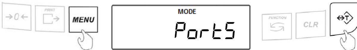
2. Choose the ports to be configured by selecting “r5232” or “USB”. Confirm the selection by pressing the T key.
