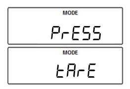
3. Place an empty vial or counting container on the pan. The container's weight will be displayed. Wait for the weight to stabilize and press the T key to tare.
