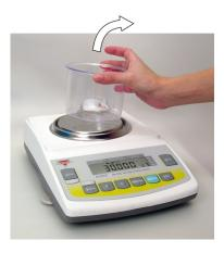
*Automatic mode:* Result will be automatically cleared; the scale will perform an automatic tare.
