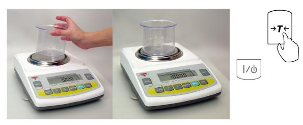
2. The scale will display the weight of a previously stored sample. To accept the current sample setting, press the "T" (YES) key and skip to step 5. To assign a new sample, press the  $\rightarrow 0 \leftarrow$  (NO) key.
