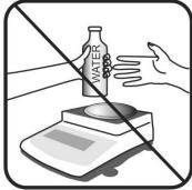
DO NOT pass or handle liquids near the torque gauge to prevent spillage and liquid damage!
