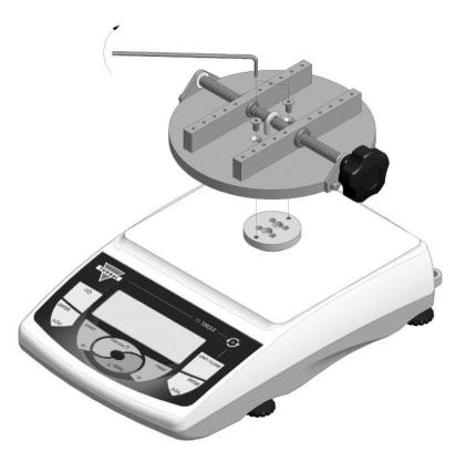
3. Install the clamping posts on the mounting rail by inserting them into the rail openings. Space the posts accordingly to diameter of the measured container.
