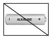
Always disable charging before installing disposable batteries Charging non-rechargeable, alkaline batteries can be hazardous and cause damage to the torque gauge.
