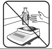
DO NOT pass or handle liquids directly over the scale to avoid spillage and liquid damage!
