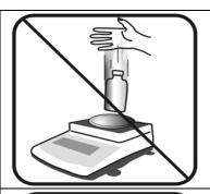
Never drop or throw any articles onto the scale's pan or onto any other parts of the unit!
