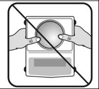
When moving the scale do not press or apply force onto the scales pan!
