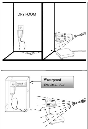
The power cord should be "fished" into a dry room or a waterproof electrical box. Consult a licensed electrician regarding an appropriate location and connection methods.
