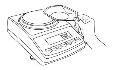
2. Place an empty container on the pan. The container's weight will be displayed.
