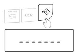
4. After the container is tared, "In9 0 I" will appear on the display, indicating the scale is ready for the first ingredient.
