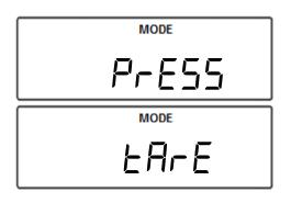
Place an empty vial or counting container on the pan. The container's weight will be displayed. Wait for the weight to stabilize and press the T key to tare.
