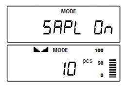
5. The scale will display the weight of the sample. Press the T key to confirm the sample weight.
