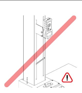
Never use the test stand if there is an object or material wedged in the column guide tracks!
