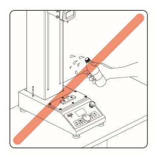
DO NOT pass or handle liquids near the test stand to prevent spillage and liquid damage!
