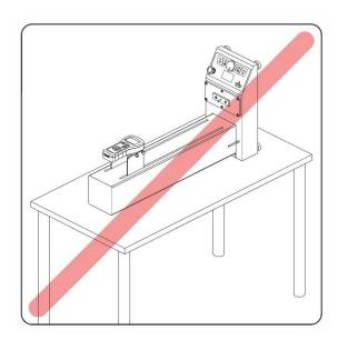
Always install the test stand in its intended orientation only!
