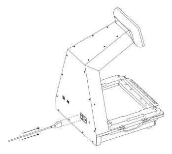
Insert the power cord into the power port located on the back of the unit and plug the cord into your wall outlet.
