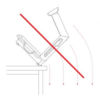
**DO NOT** pass or handle liquids directly over the pill counter to avoid spillage and liquid damage!
