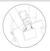
First, insert the power plug into the touchscreen display and screw it in tightly to secure it. Then, connect the USB and HDMI plugs to their respective sockets.
