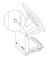
Attach the Wi-Fi antennas to the antenna ports located on the sides of the unit. Ensure the antennas are attached even if you do not intend to use a wireless internet connection.
