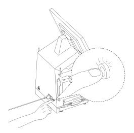
Press the power button located at the back of the unit. Wait for the VIVID Workstation to power on and initialize.
