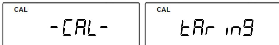
4. When prompted, load a calibration weight equal to the weight displayed on the screen. (Calibration weight varies by model).
