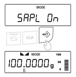
**Note**: The reference sample must be equal to or greater than 100d. Attempting to set a sample lower than 100d will result in a "*SAPL LD*" error.
