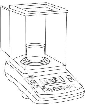
3. The scale will display the weight of the previously stored sample and the command "SALLE" sequentially. To accept the current sample weight, press the "T" (Yes) key. To change the sample weight, press the " $\rightarrow 0 \leftarrow$ " key.
