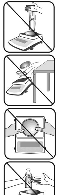
Never drop or throw any articles onto the scale's pan or onto any other parts of the unit!
