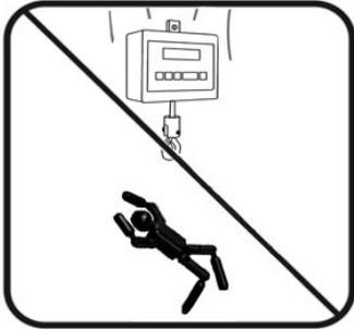
When mounting take extra caution and make sure that your mounting method will support a load which is equal to twice the weight of the scale's maximum weighing capacity. Improper mounting of the crane scale can result in having the unit fall from its mounted height and can cause serious injury or death.
