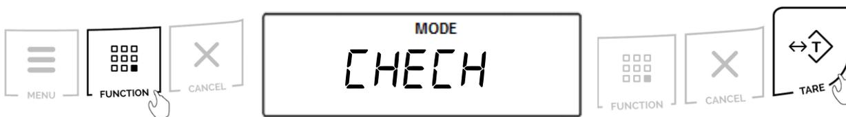
2. The current, set *UNDER*-limit and the command “*UndEr*” will appear on the display sequentially. To accept the current *UNDER*-limit, press the “T” (Yes) key. To change the limit, press the “→0←” key.
