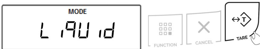
2. Options LIQUID is selected, PLUNGER "PLUNGER" will be displayed, indicating to enter the volume of the plunger used in the density kit, which can be found on the plunger hook included with the density kit.
