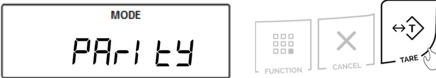
2. Choose the parity type to be used (“none”, “odd”, and “Even”). To confirm the selection, press the “T” key.
