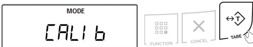
**Note:** Scrolling through the options may be accelerated by manually pressing the “→0←” (NO) key.
