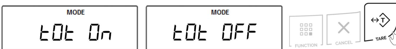
3. Totalizing can operate in three different modes: Automatic (AUTO), Semi-automatic (SE-AUTO) and Manual (MANUAL) (see Table 9.6). The three operating modes will display sequentially. When the desired mode is displayed, press the “T” key to make the selection.
