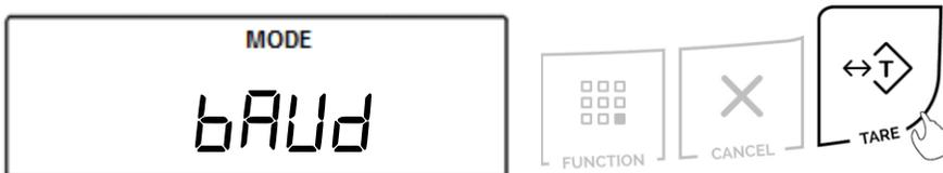
2. Choose the baud rate to be used (“1200”, “2400”, “4800”, “9600”, “19200”, “38400”, “57600”, and “115200”). To confirm the selection, press the “T” key.
