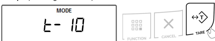
**Note:** Select longer time intervals when weighing very active animals. Longer time intervals will allow the scale to take more readings while the animal is moving on the pan and provide an accurate result.
