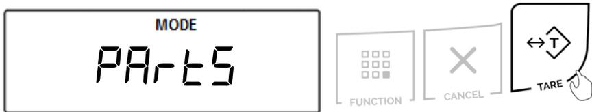
2. Commands “Co On” and “Co OFF” will be displayed sequentially. To enable Parts Counting, select “Co On” with the “T” key. To disable Parts Counting, select “Co OFF” with the “T” key.
