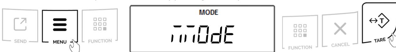
2. The scale will display available modes sequentially. When the desired mode is displayed, press the “T” key (Yes) to make the selection.
