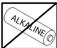
Always disable charging before installing disposable batteries
