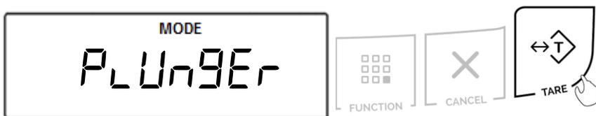
3. To key in the volume of the plunger, use the following keys: The →0← key to increment a digit, the T key to accept and go to the next digit, and FUNCTION to accept the setting.
