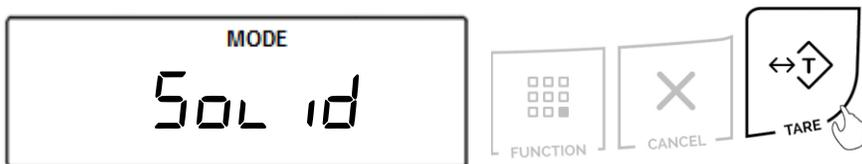
2. Options "H2O" H2O (distilled water), "EtHAnOL" ETHANOL, and "OtHEr" OTHER will scroll sequentially. Select the liquid that will be used in this density calculation by pressing the T key when the corresponding command is displayed.
