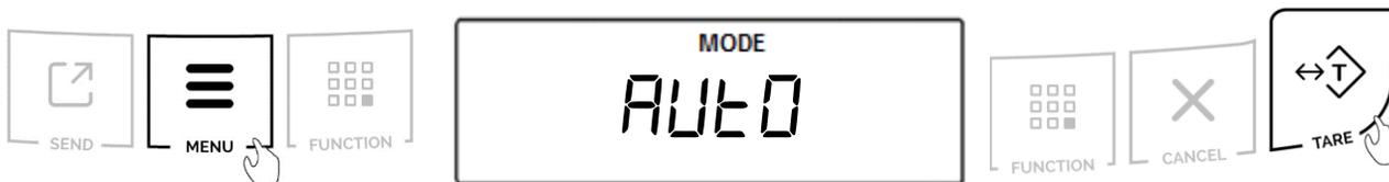
2. To enable AZSM press the “T” key when “AUTO On” is displayed. To disable AZSM press the “T” key when “AUTO OFF” is displayed.
