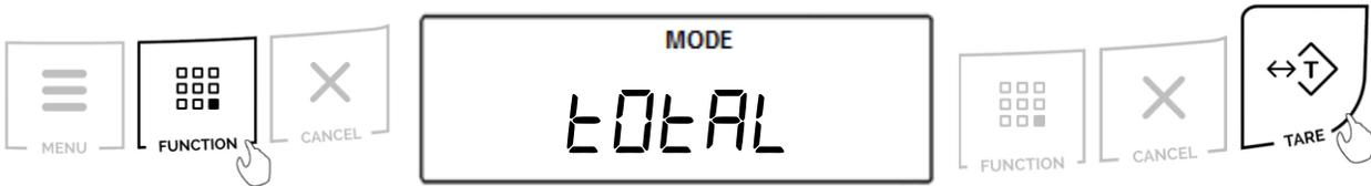
2. Place an empty weighing container on the pan. The container’s weight will be displayed. Wait for the weight to stabilize and press the “T” key to tare.
