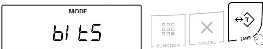
2. Choose “7 bitS” or “8 bitS”. To confirm the selection, press the “T” key.
