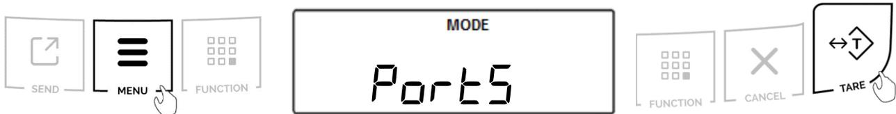
2. Choose the ports to be configured by selecting "rs232" or "usb". Confirm the selection by pressing the "T" key.
