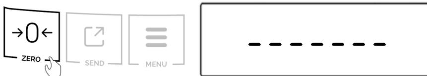
4. When finished re-zeroing, the scale will return to Weighing Mode and the display will indicate "0". A new center of zero has been set, and the scale is ready for weighing.
