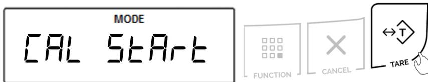
4. During calibration the scale will display “CALIB”. When calibration is finished the scale will return to weighing mode.
