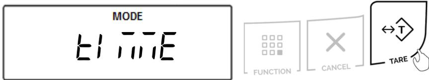
3. The current time setting will be displayed. To adjust the time press the “→0←” (NO) key.
