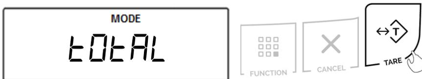
2. Commands “TOTAL On” and “TOTAL OFF” will be displayed sequentially. To enable Totalizing, select “TOTAL On” with the “T” key. To disable Totalizing, select “TOTAL OFF” with the “T” key.
