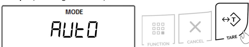
4. Once the desired operating mode for animal weighing has been selected, the scale will display time intervals for the animal weighing process, sequentially. The intervals are: 3 seconds (*t- 3*), 5 seconds (*t- 5*), 10 seconds (*t- 10*), and 15 seconds (*t- 15*). Select a time interval by pressing the “T” (Yes) key.
