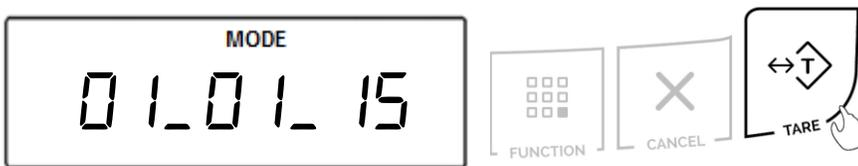
4. Use the →0← key to change minutes and hours. Press the T key to advance and confirm the time setting.
