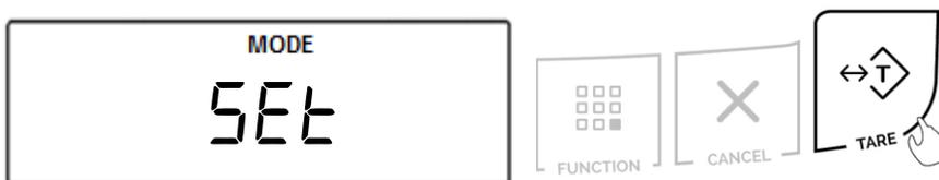
3. To enable GLP, press the “T” key when “On” is displayed. To disable GLP, press the “T” key when “OFF” is displayed.
