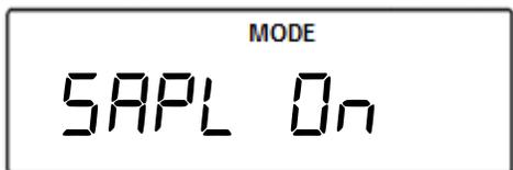
**Note:** Minimum individual piece weight must be equal to or greater than 3e. Attempting to set an average individual piece weight which is lower than 3e will result in a Sample Low Error (SAPL LD). To see this limit expressed in grams turn to detailed specifications in Chapter 2.
