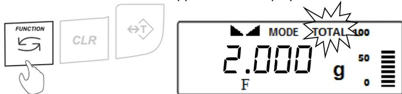
**Note:** With each added weight, the grand total result will appear on the display for approximately three seconds. To recall the grand total at any time, press the “MENU” key.
