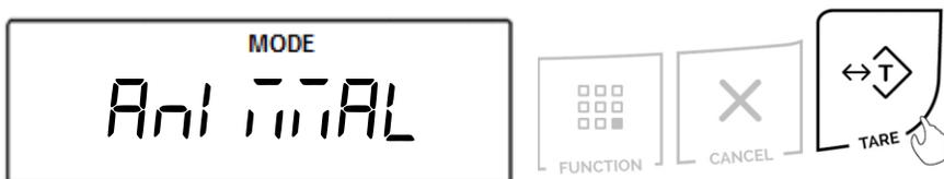
2. Commands “An *On*” and “An *OFF*” will be displayed sequentially. To enable Animal Weighing, select “An *On*” with the “T” key. To disable Animal Weighing, select “An *OFF*” with the “T” key.
