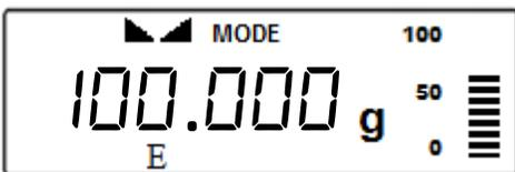
**Note:** The reference sample must be equal to or greater than 100d. Attempting to set a sample lower than 100d will result in a “SAPL LO” error.
