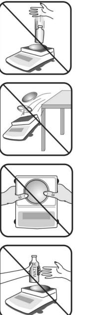
Never drop or throw any articles onto the scale's pan or onto any other parts of the unit!
