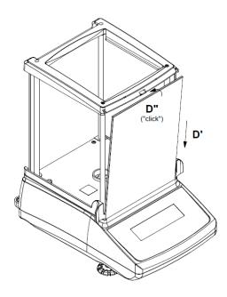
7. Insert the top chamber glass access door by sliding in the rear edge of the glass onto the chamber top frame. (E')
