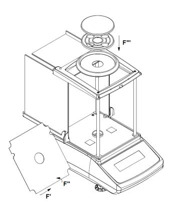
6. Install the front-chamber glass by inserting the bottom edge into the scale housing (D') and securing the top edge in the chamber top frame (D'').
