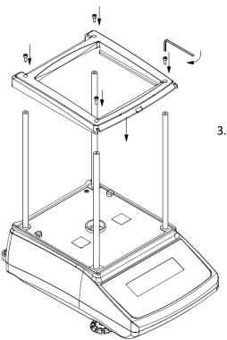
Place the chamber top frame on the posts and firmly secure it in place by screwing in the post crews with the provided wrench.
