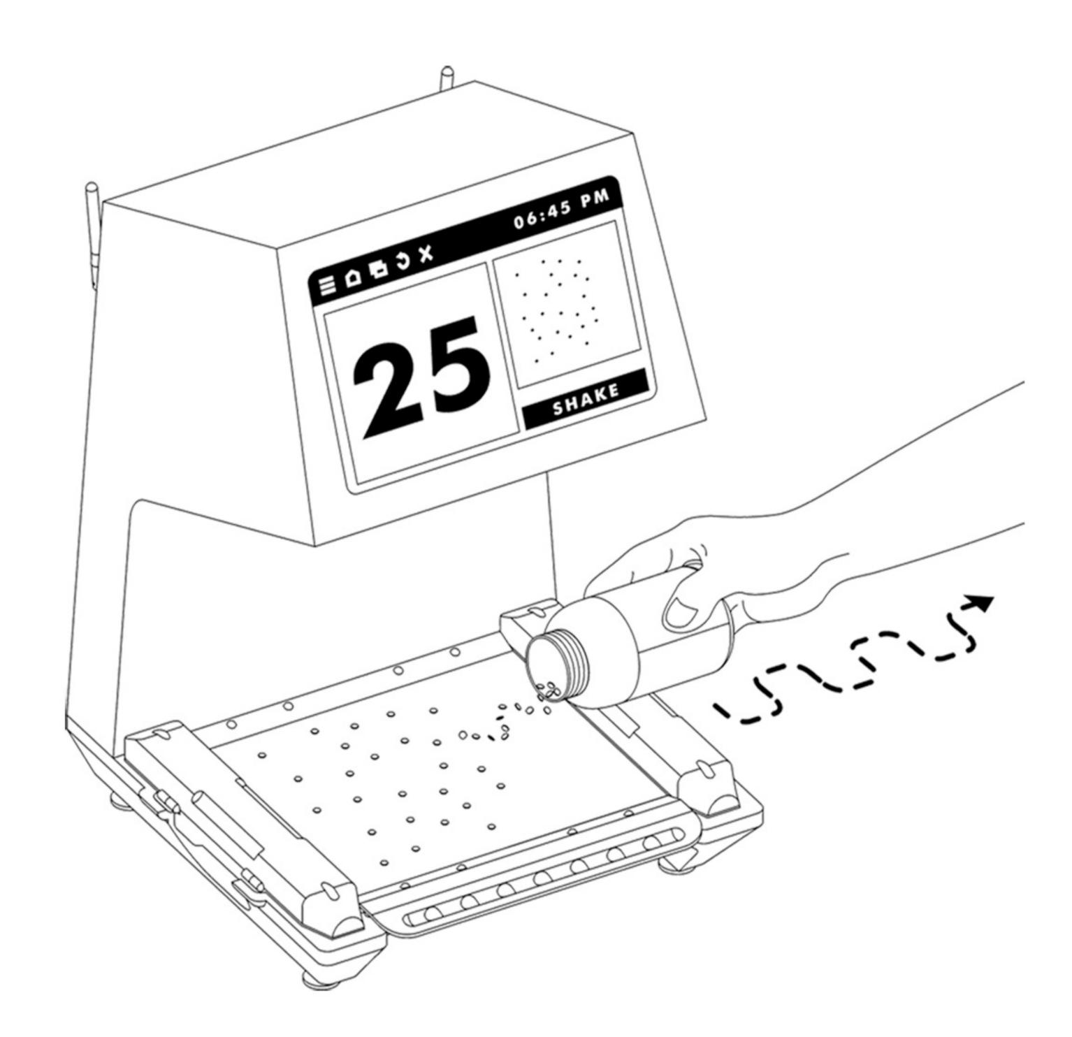
Once the pills are scattered on the tray, use the front tray handle to lift the tray up and down, and tap to assure pills spread away from each other.
